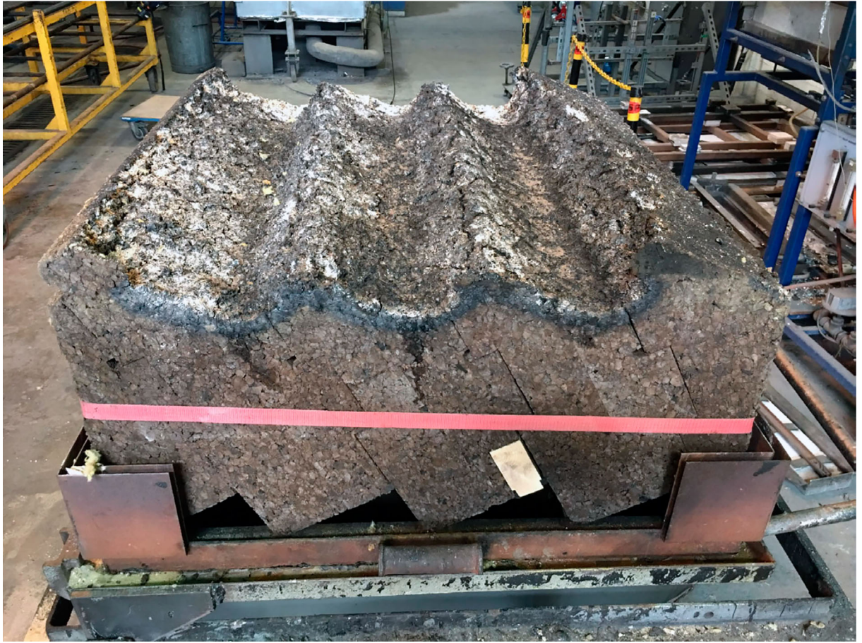
Figure 6. Sample roof panel laid horizontally immediately after fire penetration testing, with charring indicating the visible extent of fire penetration, © Matthew Barnett Howland
