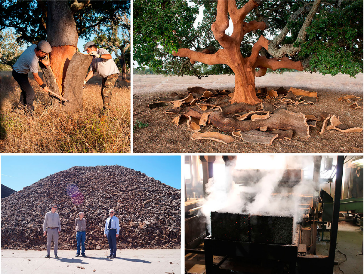
Figure 1. (top) Stripping cork from a tree in the Portuguese Montado, © Amorim; (bottom) waste cork manufactured into expanded cork billets at Amorim, Portugal, © Oliver Wilton and Matthew Barnett Howland
