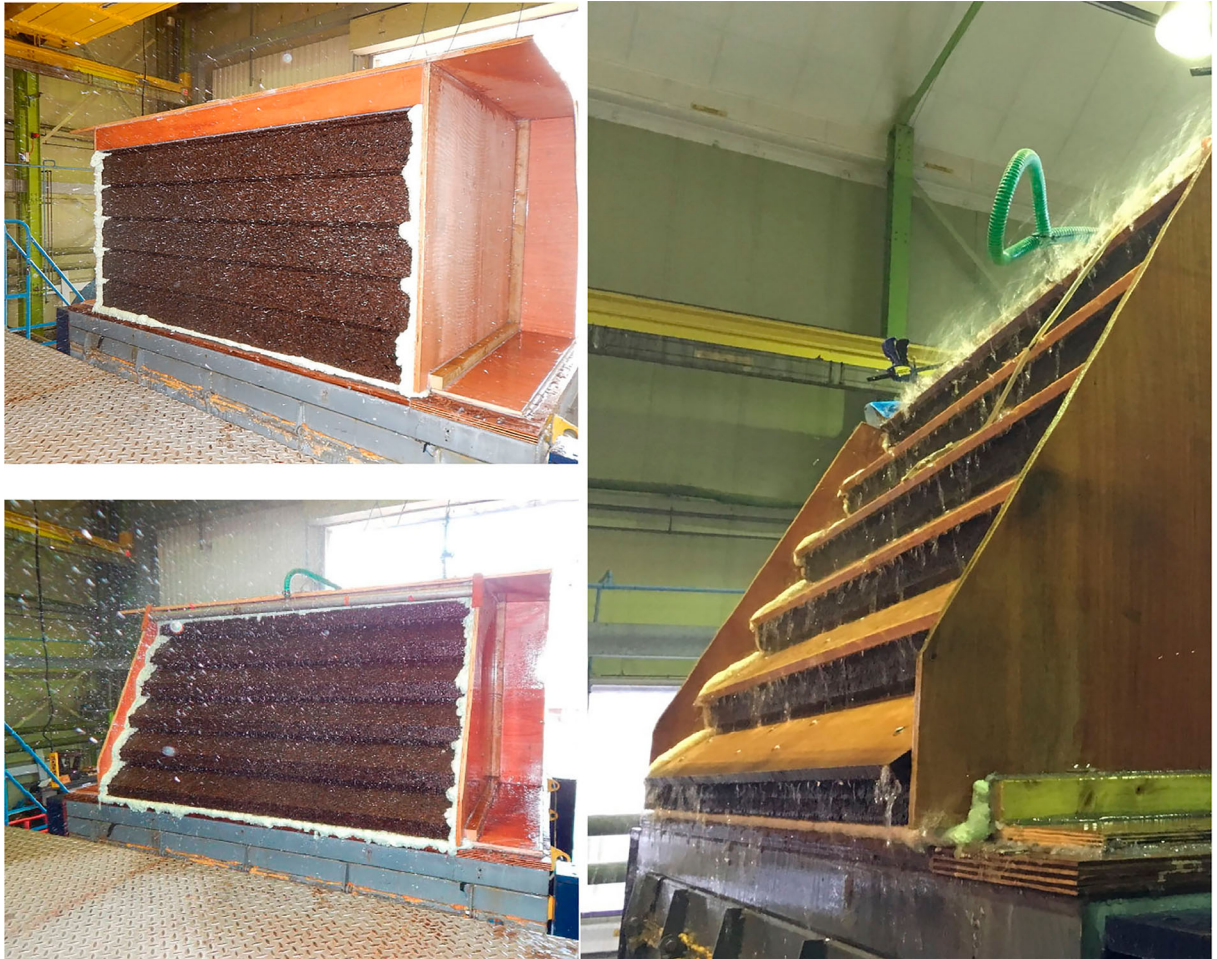
Figure 7. (top left) Wall panel under wind-driven rain testing; (bottom left) testing the first roof panel, which leaked; (right) testing the second roof panel, which didn't leak. Water shedding from timber weatherboards is visible, © Oliver Wilton and Matthew Barnett Howland
