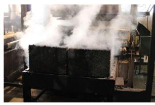
cork block assemblies, dry jointed with no glue or mortar, would provide structural enclosure, thermal and acoustic insulation, and rain and air tightness. This work was undertaken in three interrelated and overlapping stages, with initial hypothesising and prototyping being undertaken from 2014 to 2015, the major research project being undertaken from 2015 to 2018 and Cork House being constructed from 2017 to the start of 2019.
